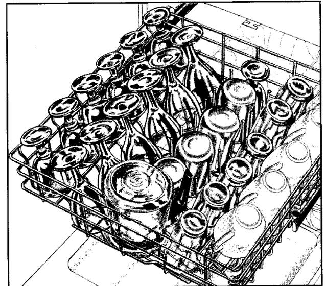
The upper rack may be removed if desired. Push inward on the front of the rack rail ends to unsnap. Remove rail ends and pull out rack.
