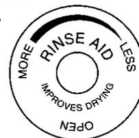
The clear indicator in the center of the cap changes from dark to light when the reservoir is nearly empty. This indicates that it is time to refill the dispenser.
